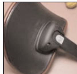
7. View of completed backrest which is ready to be attached to the upright on the stool's mechanism
